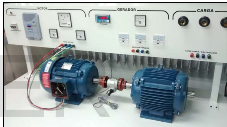
Figure 10 – Proposed bench in final phase of assembly
